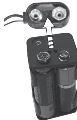
4. Replace the batteries with 4 AA **alkaline** batteries.
