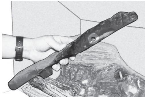
**Note:** Make sure the lower end of the top log rests on the front log as indicated and does not fall below in the firebox.
