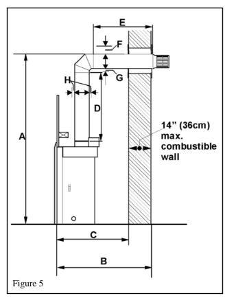
For installations with a horizontal rear termination, the combination of horizontal and vertical vent pipes must be within the allowed area shown in Graph 1. A minimum vertical pipe run of 6" is necessary.
