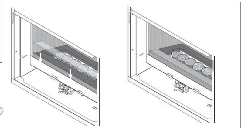
6. Place the left twig across the second and third rocks from the **left**; rest its end on the glass near the edge of the platform as shown. **Make sure to leave a gap between the twig and the first rock to allow flame to come up between the twig and the rock.**
