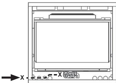
**If the circulating fan is to be installed, be aware that the supply pipe run inside the case should be at the same height as the appliance inlet pipe in order to clear the fan. If intending to fit an internal isolating valve, check that it will be clear of the fan.**
