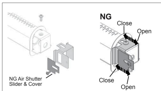
In a few unusual installations, the flame picture may be improved by adjusting the aeration. The need for adjustment should be determined only by operating the appliance with the ceramic rocks and window installed.
