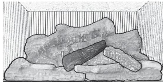
6. Identify the left cross log; it has a hole under its narrow end. Place its narrow end on the pin located on the rear log. Rest its wider end on the crook in the front left log at an angle of approximately 30 degrees from the center line of the fireplace to allow for the flame to come up in front of the rear log.
