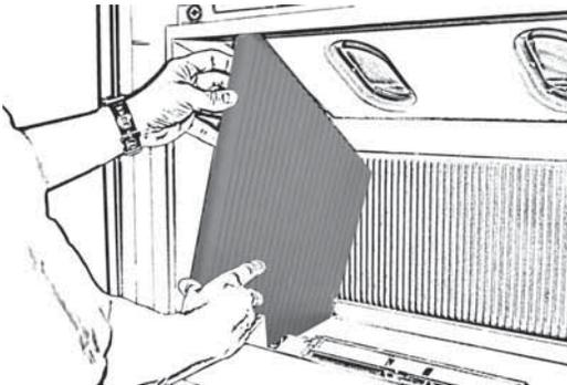
3. Hold the right hand side panel at an angle and insert its bottom edge inside the firebox. Rotate the panel to a vertical position ensuring that the top edge is behind the flange of the firebox. Pull the panel as far forward as possible against the right edge of the firebox.
