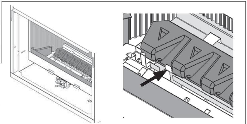
3. Install the ceramic platform in the firebox rotating down to insert the front first behind the Front Support. Lay the back of the ceramic platform against the rear ceramic panel again being careful not to scrape the ceramic panels.
