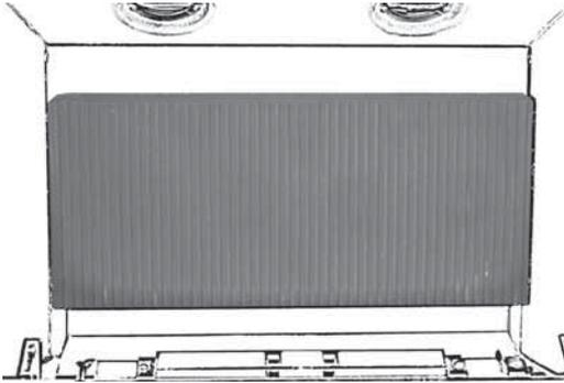
2. Hold the left hand side panel at an angle and insert its bottom edge inside the firebox. Rotate the panel to a vertical position ensuring that the top edge is behind the flange of the firebox. Pull the panel as far forward as possible against the left edge of the firebox.
