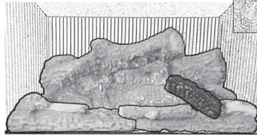
5. Identify the middle cross log. It does not have a hole underneath. Place its narrow end on the flat depression in the rear log next to the right cross log on the rear log. Place its wider end on the front log.
