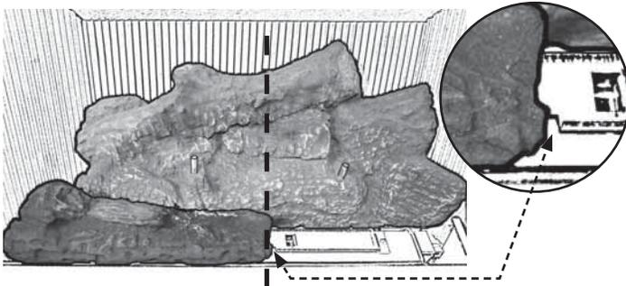
3. Place the front right log on the top of the burner with its left end abutted to the front left log and its front edge resting slightly on the window frame. **Center the front logs side to side in relation to the firebox.**
