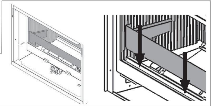
2. Place the rock ceramic base on the log support behind the burner. The front bottom of the base must rest against the vertical tab of the spacer brackets.
