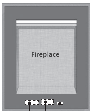
Receiver Gas Batteries valve
