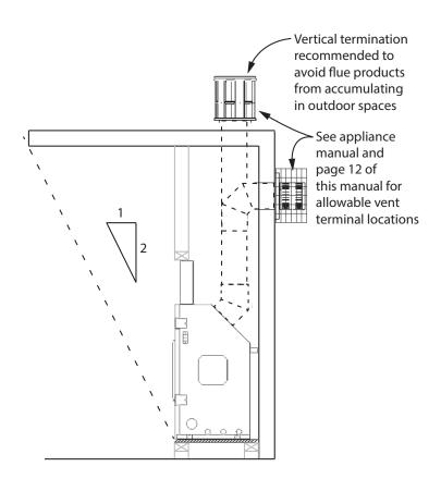
Min. required overhang Outdoor fireplace Min. required weatherproof overhang in front and at sides of installed in weatherproof fireplace is 1/2 of the height of the overhang measured enclosure from the base of the unit . 1265WSK Wall switch or **RBWSK Remote battery** & wall switch kit must be located within weather protected area Min. required overhang
