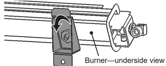
4. Transfer the burner support brackets to the new conversion burner securing them with the 2 nuts removed in step 3. **Note: do not overtighten the nuts to avoid breaking the studs.**
