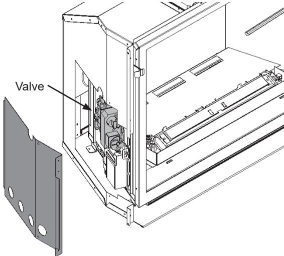
2. Fit a manometer to the manifold pressure test tap on the valve—see figure at right. Turn on the gas supply.
