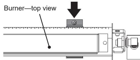
3. Detach the burner brackets from the burner by removing 2 nuts using a 5/16" (8 mm) wrench.
