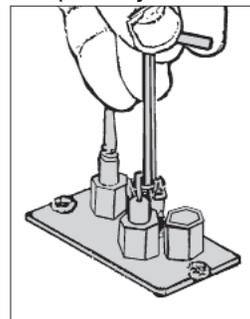
3. Replace with the appropriate pilot injector—see *Specifications* table on page 1. Screw the new injector.
