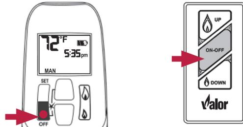
If the flames or pilot are on, they will go out and you will hear the valve motor wind down. You will hear a clunk and a beep indicating that the valve has received the signal from the remote control.
