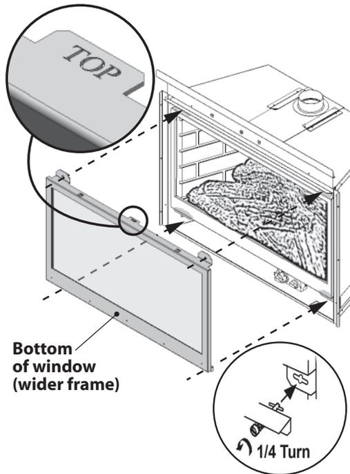
2. While you hold the window, push in and turn the two bottom spring-loaded bolts a quarter turn to engage their pin into the firebox's tabs.
