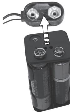
5. Replace the batteries with 4 new AA 1.5V **alkaline** batteries. Do not mix new and used batteries.
