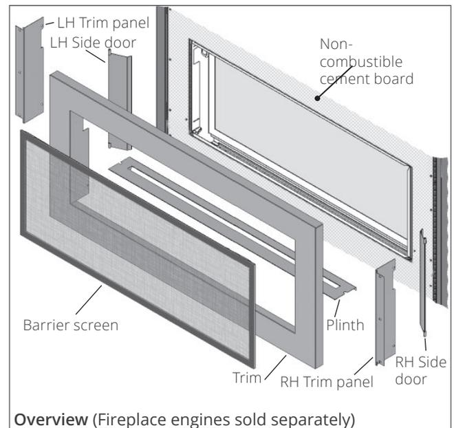
The 1550v2 Linear 3-1/2" Surround Kit is designed to be used on the Linear L1 1500 and Linear L1 2-sided 1600 Valor heaters.
