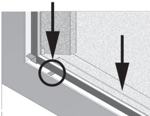
3. Verify that the screen is properly hooked to the trim and secure.
