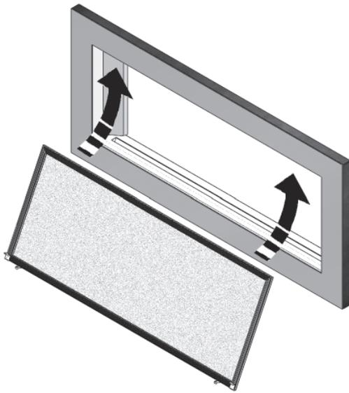
2. Grab the finger tabs on the bottom of the frame and lower the screen straight down locating the bottom hooks into slots hidden just behind surround plate.
