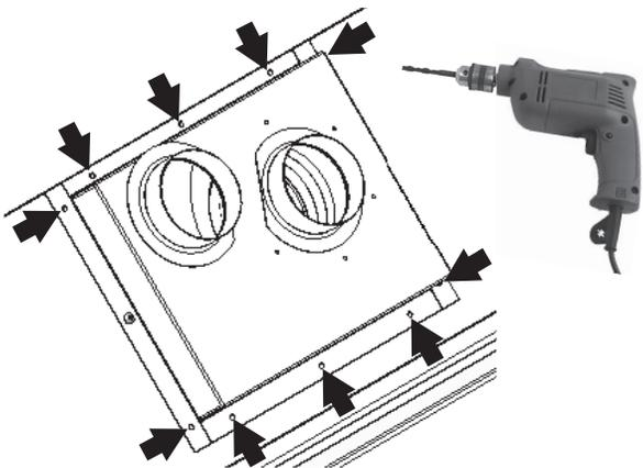
4. Re-use the 6 screws removed from the takeoff elbow to plug the unused screw holes for the 4" diameter collar around the exhaust port of the adapter. Ensure all screws are tight.
