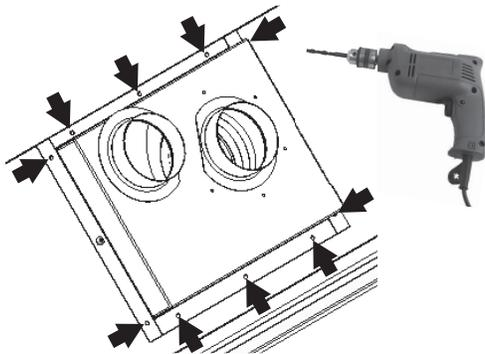
4. Fit the 4" gasket and the 4" exhaust collar over top of the 3" exhaust outlet. Fix the collar with 6 screws removed from the takeoff elbow. Ensure all screws are tight.
