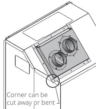
5. Connect 3" dia. flex liners directly to their respective adapter collars using hose clamps (included) and 2 sheet metal screws per liner. Refer to appliance's installation manual for the remainder of the venting installation.
