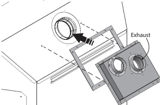
3. Pierce the remaining screw holes through the holes on the adapter box using a 1/8" drill bit. Secure the adapter box to the heater using 10 sheet metal screws provided.
