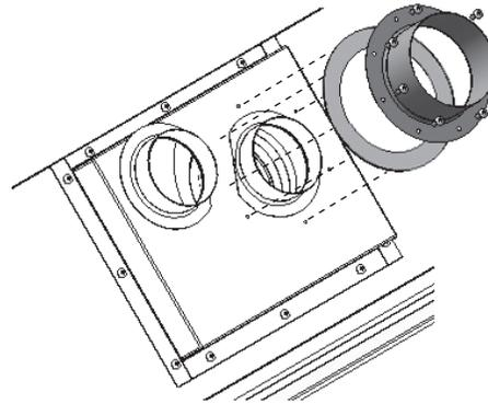
5. Connect a 3" diameter intake and 4" diameter exhaust flex liner directly to their respective adapter collars using the hose clamps (included) and 2 sheet metal screws. Refer to the appliance's installation manual for the remainder of the venting installation.
