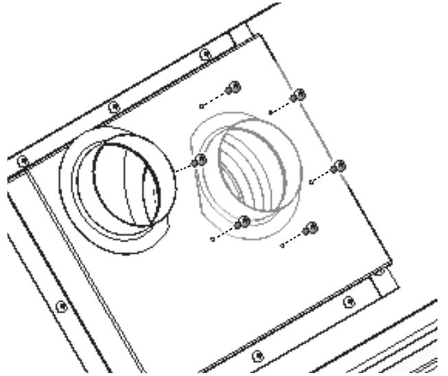
**NOTE:** On the 200 models, one corner flange of the adapter extends over the edge of the appliance's outer case, once installed. You can cut away or bend down this flange.
