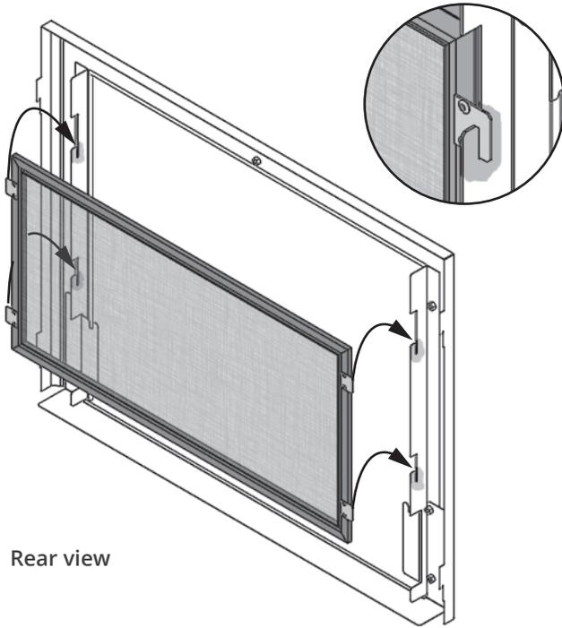
6. **738 only.** Clip the extension baffle provided with the Clearview frame to the sheet metal edge of draft hood divider as indicated.
