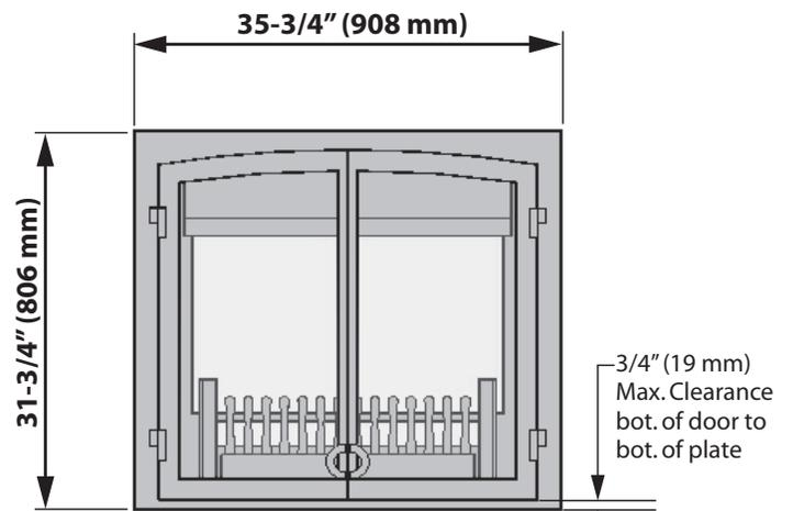
**\*NOTE:** Bottom of plate is flush with bottom of heater. Install bottom of heater flush with finished hearth.
