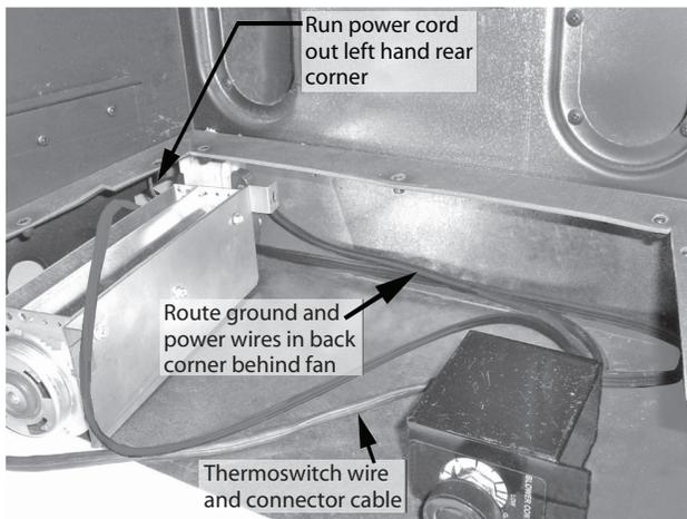
4. Fit the fan unit by placing it into the rear of the liner box (with the wires running behind) and secure to the rear wall using the two screws provided.
