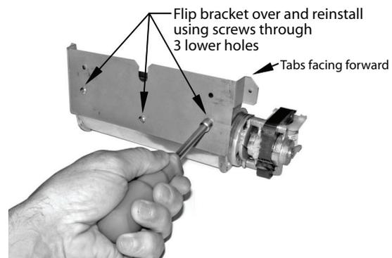
2. With the burner module removed, install the fan unit into the rear convection channel on heater.
