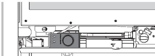
2. Install the thermostat to the underside of the burner plate, behind the pilot area, with 2 screws taken from the burner plate.
