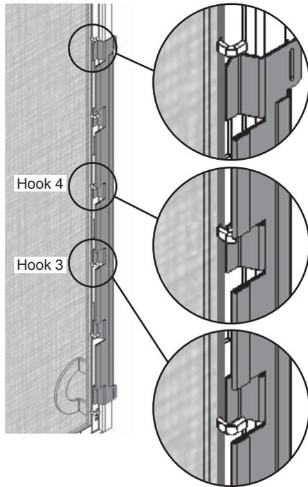
5. Holding the door frame shield, bend top and bottom tabs around the edge of the door frame flange to maintain it in place.
