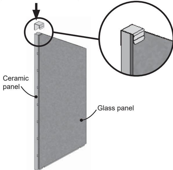
9. Place the clipped side panels on the support of the corresponding side in the firebox.
