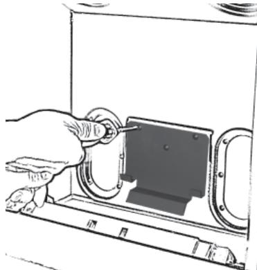
2. Install the kit's rear panel bracket on the panel's support just installed. Slide the rear panel bracket on the screw and push it down against the bottom lip of the panel support. Tighten the screw.
