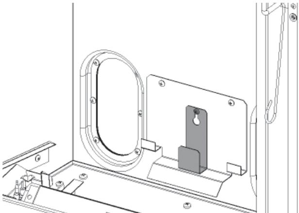
3. Back off the rear screw of one of the side wall supports. Slide the side bracket supplied with the kit on the screw, push it up against the underside of the side wall support and tighten the screw.
