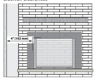
**Minimum** distance from side of appliance (liner box) to combustible wall: 4" (102 mm).
