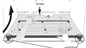
3. To reinstall the burner, fit the burner in the firebox inserting the front tabs first in the lances.
