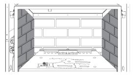
5. Tighten the side panel anchors on each side of the firebox.
