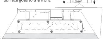
3. Place emberbed cover over front of burner with tabs into recess part.
