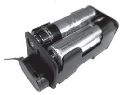
On the left hand side of the firebox, pull the loose wire that is already connected to the receiver and connect it to the battery holder. Place the battery holder to the left of the firebox, in front of the receiver.
