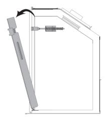
3. Lift the window out of its bottom railing and set it aside in a safe place to avoid damage.
