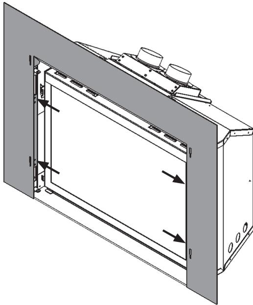
3. The backing plate is now ready for a front to be installed onto it. See the installation manual for your trim for instructions.
