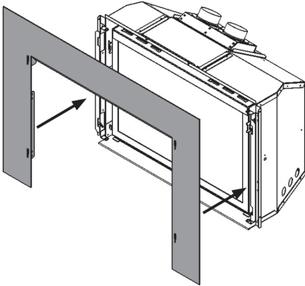
2. Attach the plate using 4 screws into the left and right sides.
