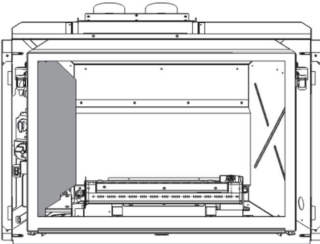
4. Place the rear filler panel on the bottom railing against the rear firebox wall.
