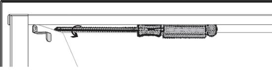
2. Rotate the anchor out of the way, and slide the left hand side filler panel against the firebox left side.
