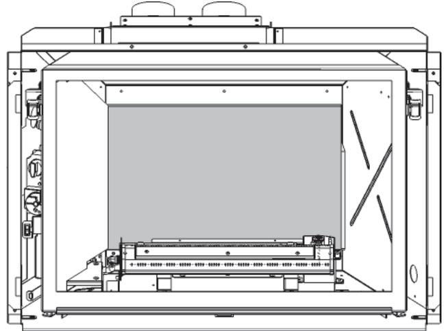
5. Place the rear glass panel, smooth side visible, on top of the filler panel. Slide the panels behind the left hand side panel.
