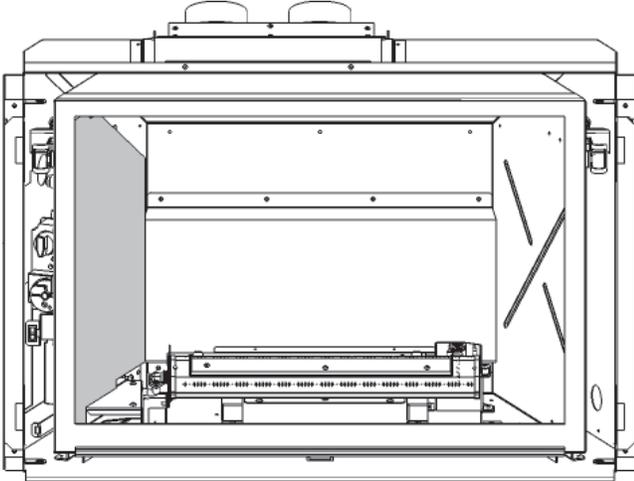
3. Place the left hand side glass panel, smooth side visible, on top of the filler panel and rotate the anchor back down to hold the panels.
