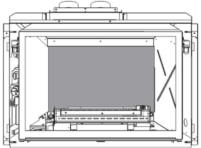
6. Place the top panel on top of the left hand side and rear panels.
