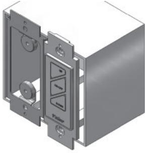
10. Place and secure cover plate to box using 4 screws provided.
