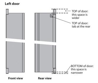
7. Insert the left hand door top hinge pin in the hole at the top of the CIK frame, then the bottom hinge in the hole of the cover panel. Turn the door in toward the back of the fireplace.
