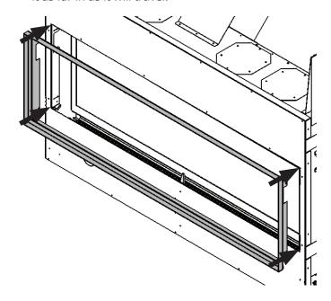
4. Screw the CIK frame to the interior of the opening (4 screws).
