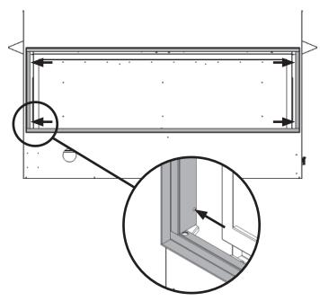
The fireplace and kit are now ready for wall finishing to take place. Cement board, tile, or other wall finishes may be completed right up to the outer edge of the CIK frame. Do not finish past this edge, as it will prevent barrier screen installation.
