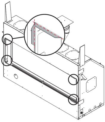
2. File or trim any remaining sharp edges. Be careful not to allow material to fall into the appliance.
