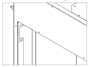
3. Slide CIK frame into the opening as shown, pushing it as far in as it will travel.
