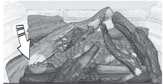
Pilot Flame can be seen on the left side of the fuel bed
