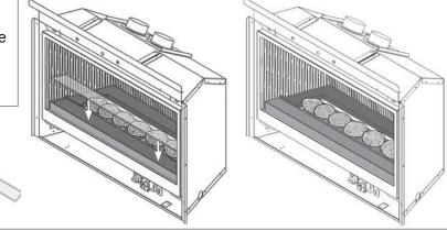
Place the left twig across the second and third rocks from the left; rest its end on the glass near the edge of the platform as shown. *Make sure to leave*
