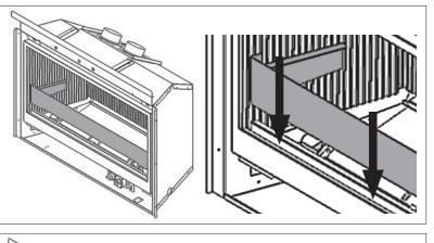
2. Place the rock ceramic base on the log support behind the burner. The front bottom of the base must rest against the lip of the support.
