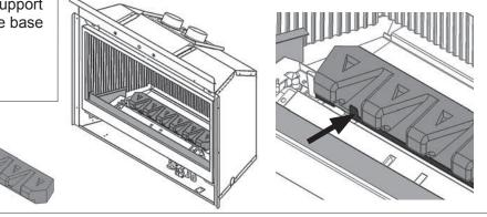
Install the ceramic platform in the firebox rotating down to insert the front first behind the Front Support. Lay the back of the ceramic platform against the rear ceramic panel again being careful not to scrape the ceramic panels.
