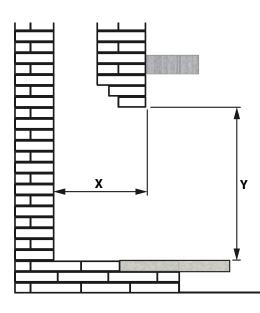
Check that masonry step does not interfere with install dimensions or vent pipe.
