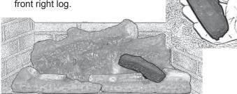
Identify the middle cross log. It does not have a hole underneath. Place its narrow end on the flat depression in the rear log next to the right cross log on the rear log. Place its wider end on the front log.
