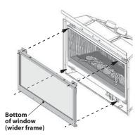
3. Push in the top of the window against the firebox and fasten the two top spring-loaded bolts a quarter turn.
