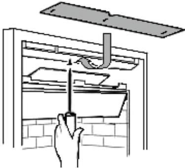
3. Mount 4 hinge pins to steel backing plate and install backing plate as shown using screws provided.
