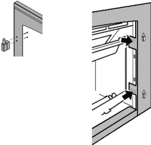
4. Clip in left and right side trim pieces. Adjust tabs by bending to fit if necessary.
