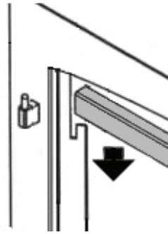
6. Drop doors onto hinge pins.
