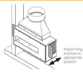
Fit the blower to the wall studs securing it through the brackets with wood screws. The universal boot may either go upward or downward. It comes oriented towards the back of the blower. This can be changed if desired. The universal boot may also be removed for connection directly to a wall stack.
