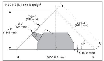
\*Not compatible with 1400M except when using HeatShift LDK1 or LDK4 Plenum
